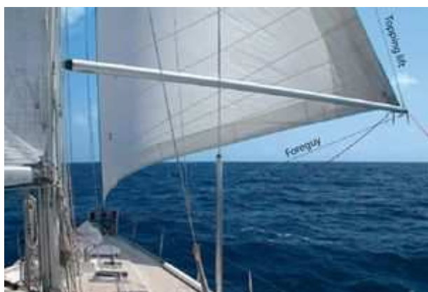
Example of a common configuration for a pole set to windward for sheeting a headsail.
